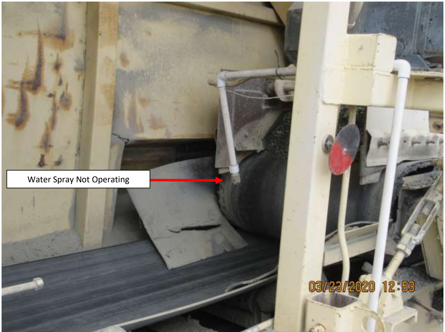
Photo 1 – Air Pollution Control Not in Operation
