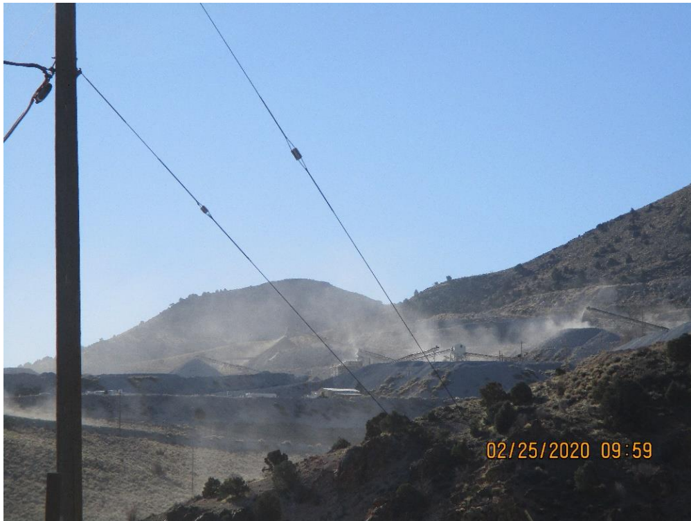
Photo 2- Water Sprays Not Operating
