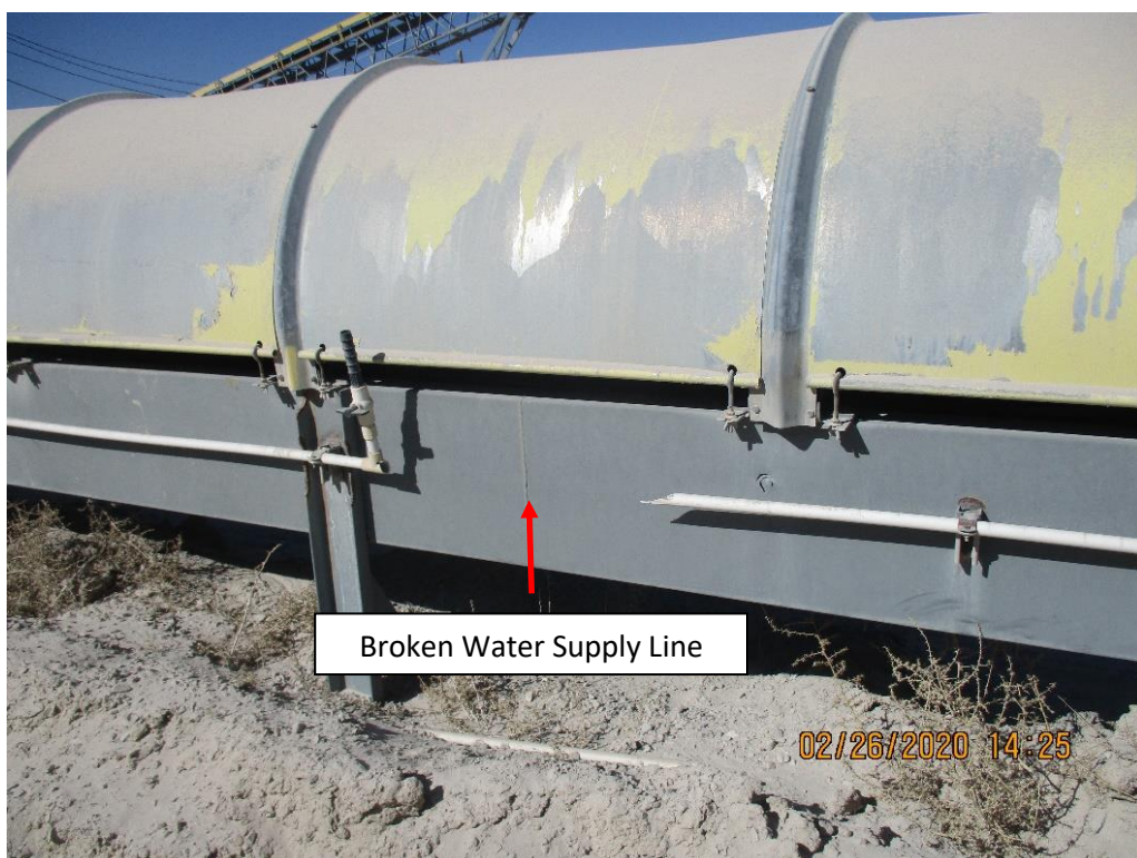
Photo 4 – Another Example of Water Sprays Not Operating
