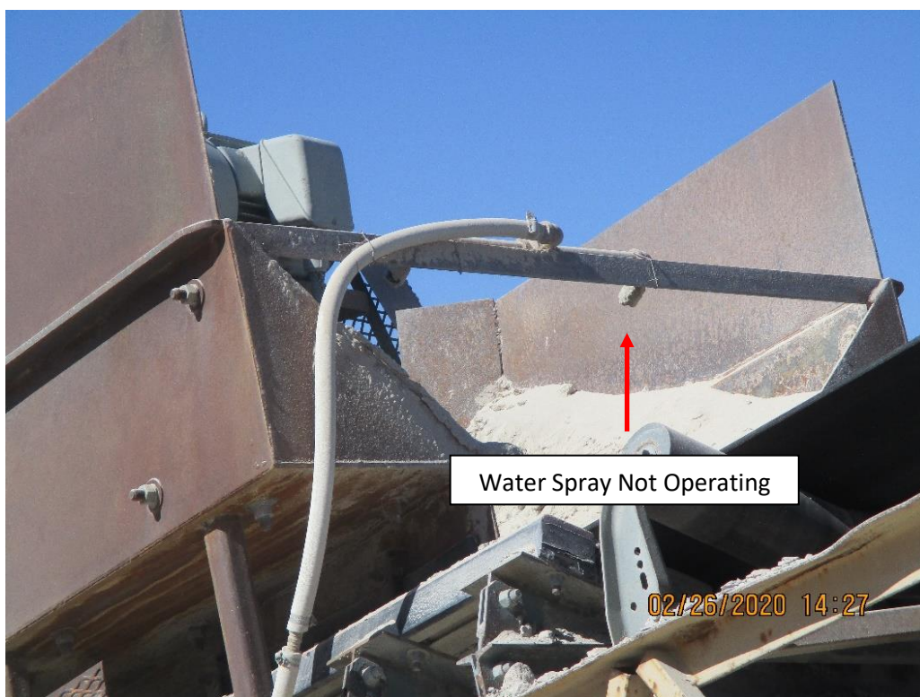
Photo 4 – Another Example of Water Sprays Not Operating
