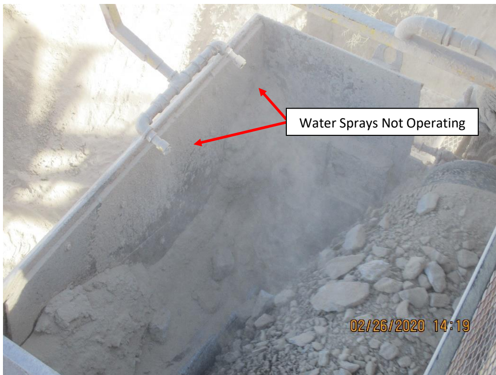
Photo 2- Water Sprays Not Operating
