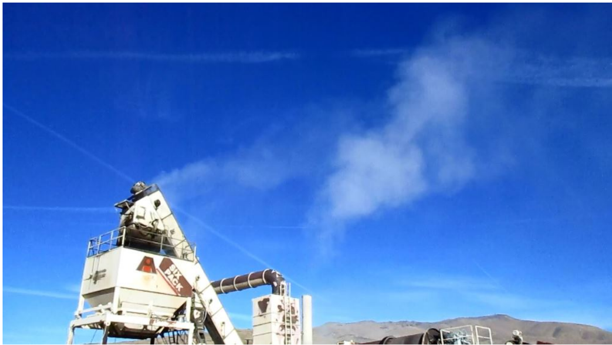
Photo 2: During visible emission observation showing average opacity of 37.3%. (image from BAPC video on October 20, 2016).
