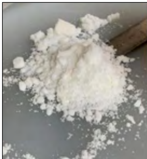
Figure 11: \text{MgSO}_4 \cdot 6\text{H}_2\text{O} crystals generated during continuous testing
