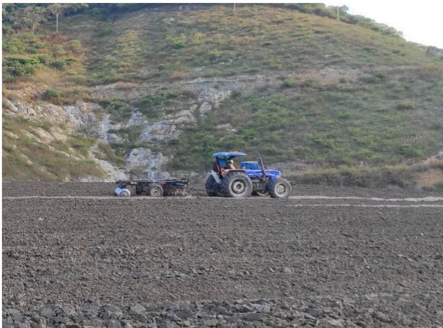
Figure 1 – Scarifying Tailings for Drying
