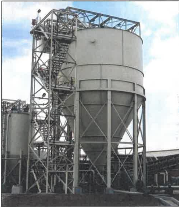
Figure 3.4 Ultra High Rate Thickener (Deep Cone Paste Thickener) (EIMCO E-CM™ - Jewell and Fourie 2015)
