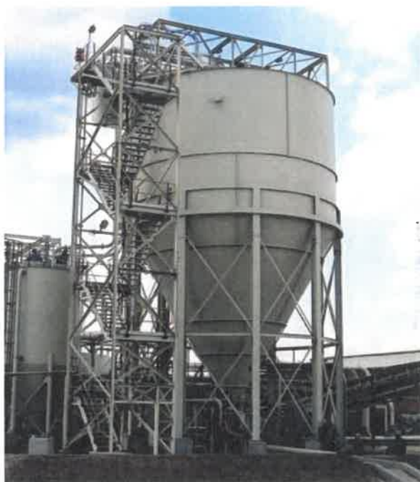
Figure I-3 Ultra High Rate Thickener (Deep Cone Paste Thickener) (EIMCO E-CM™ - Jewell and Fourie 2015)
