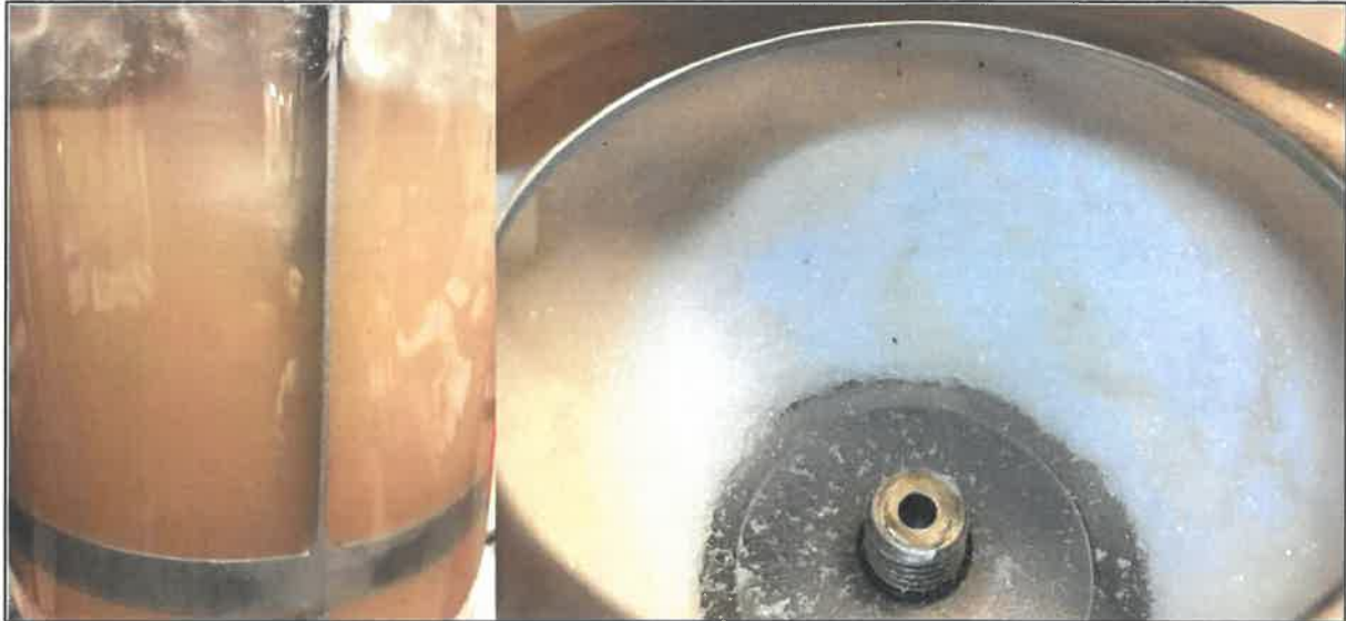
Figure 10: a) \text{MgSO}_4 \cdot 6\text{H}_2\text{O} crystal slurry, b) after centrifuge, crystal separation
