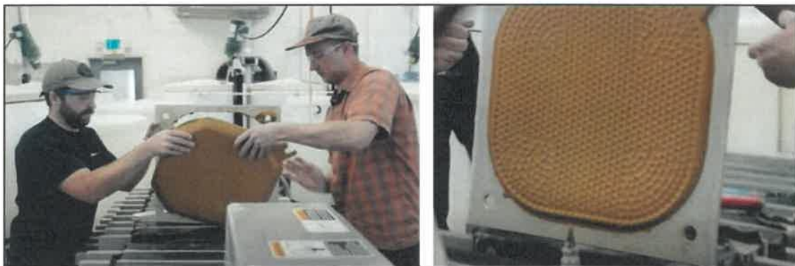
Figure 2: Photos of filter cakes directly out of filter press
