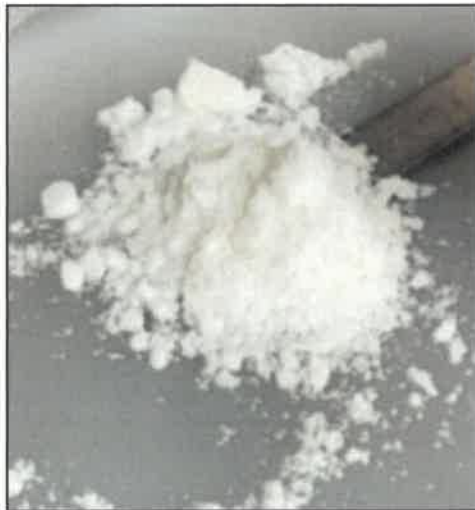
Figure 11: \text{MgSO}_4 \cdot 6\text{H}_2\text{O} crystals generated during continuous testing
