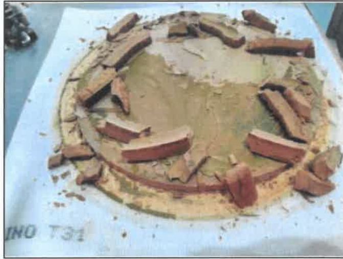
Figure 4: Filter cake from Vendor 1 test
