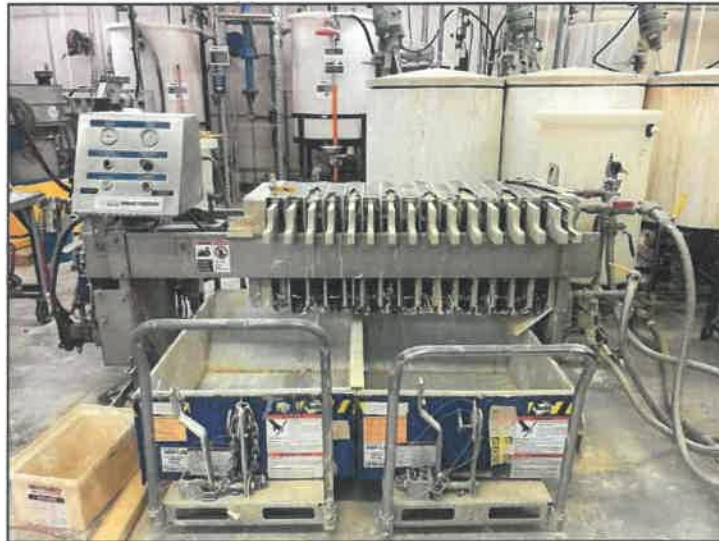
Figure 1: Pilot scale plate and frame filter press
