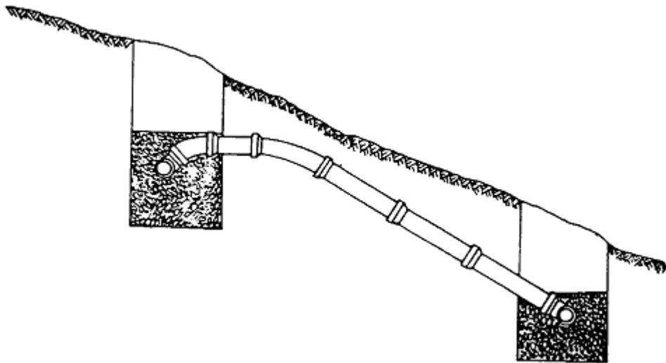
Sec. 79. 1. *Except as otherwise provided in subsection 2, a capping fill trench may be used where conditions relating to high groundwater prohibit the installation of an absorption trench pursuant to section 75 of this regulation.*
